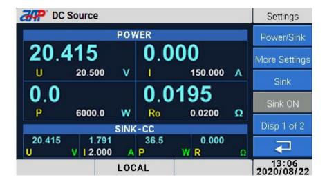
According to the actual test requirements, the working CC current under the sink mode can be adjusted to effectively absorb the back electromotive force and make the voltage curve smoother.
